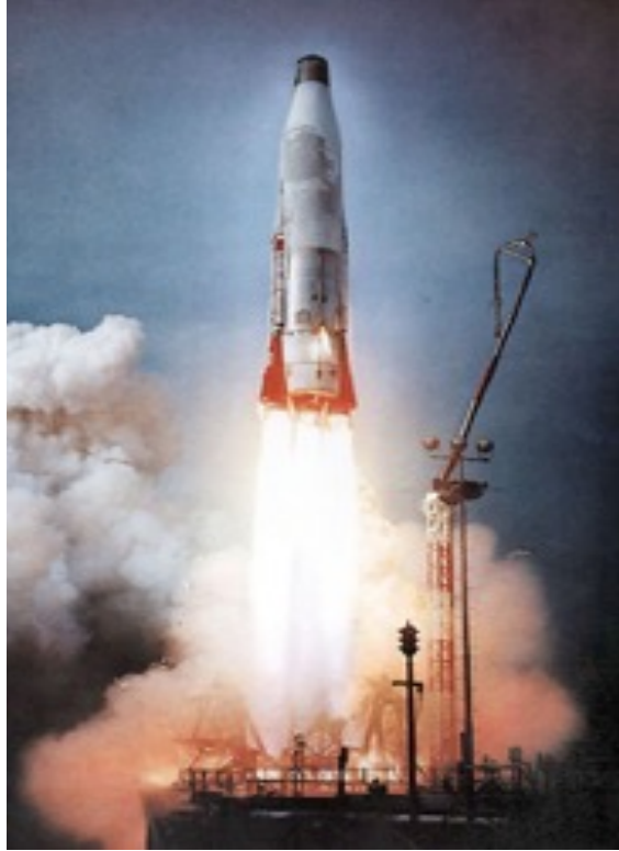
(Figure 6- Atlas rocket with Mark 2 Reentry vehicle installed)
