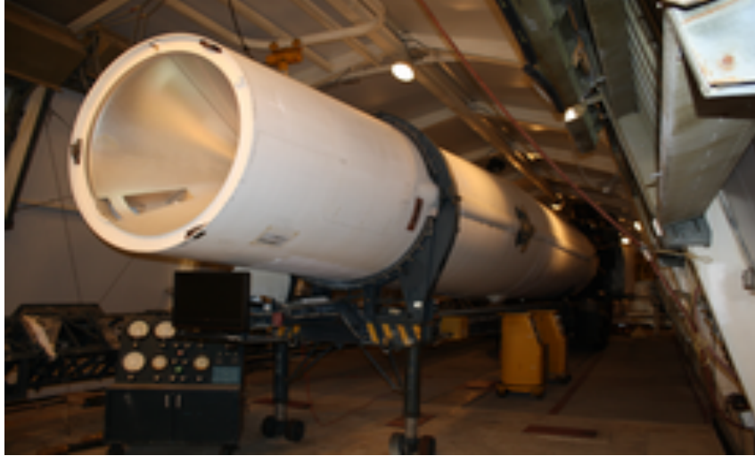
(Figure 4- Thor rocket illustrating the Mark 2 Reentry vehicle insertion point)
